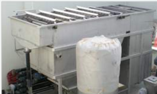
DAF equipment is an all-in-one equipments with DAF tank, surface scraper, DAF pressure tank and high pressure pump.
